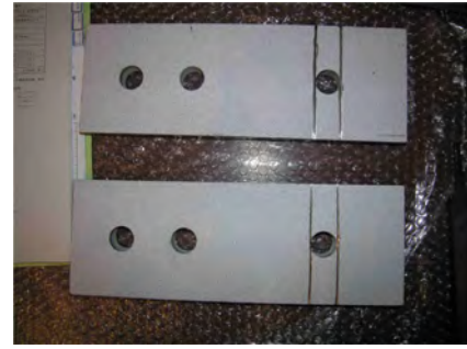
Figure 24. Flawed test articles: Direction orthogonal to force application.
