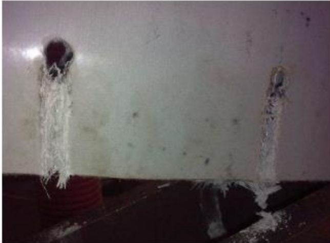
Fig. 14 Experimental research on GFRP. Bolted connections. Fig. 15. Axial load test on GFRP pannels
